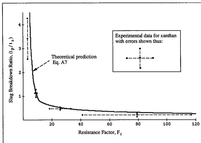
Figure 15: Comparison of experimental and theoretical dimensionless slug breakdown ratio for viscous fingering through xanthan slugs in layered systems; Eq. A7 with  $\omega = 2/3$ , Pack 2,  $k_1/k_2 = 11.2$ , see data in Table 4.
