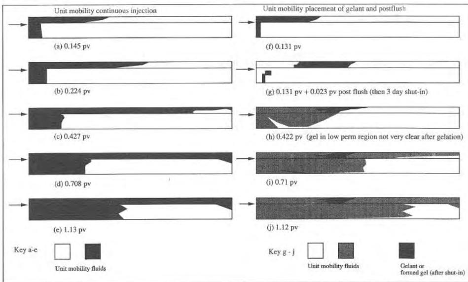
Figure 8: Experimental comparison of a unit mobility continuous displacement with a corresponding unit mobility gelant treatment using a model fluid system which subsequently sets in the pack (see text);  $k_1/k_2 = 5$ ; (Pack 3; Table 1).
