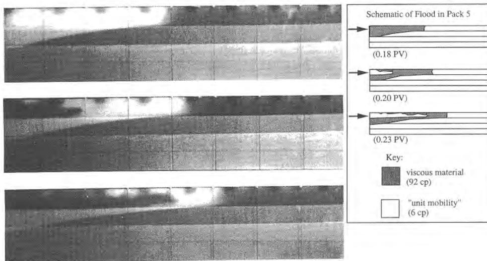
Figure 11: Images from the viscous slug placement in Pack 5 (Table 1) with  $F_r = 15.3$ ; interpretation shown inset.
