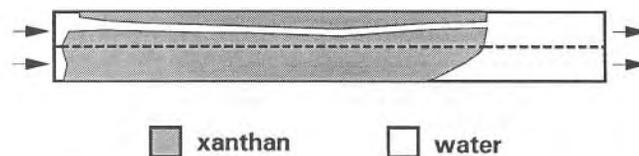
Figure 7: An example of the fingering of water through a bank of 2000 ppm xanthan; fingers form in the high permeability layer (Pack2; Table 1).
