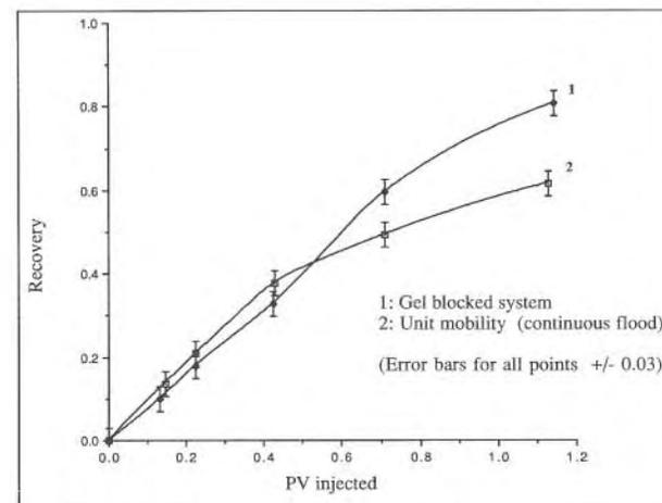
Figure 9: Recovery vs. total pore volume injected for the experimental floods in Fig. 8 comparing the recovery for a gel treatment with that of the "untreated" system in a unit mobility continuous displacement
