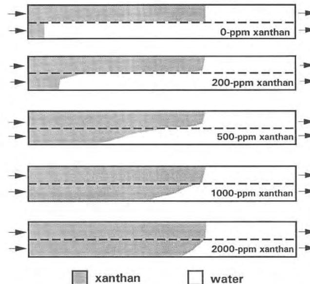
Figure 5: Crossflow in a two layer bedpack during displacement of water by xanthan solutions;  $k_1/k_2 = 11.2$ ;  $F_r$  = varying (Pack 2, Table 1).
