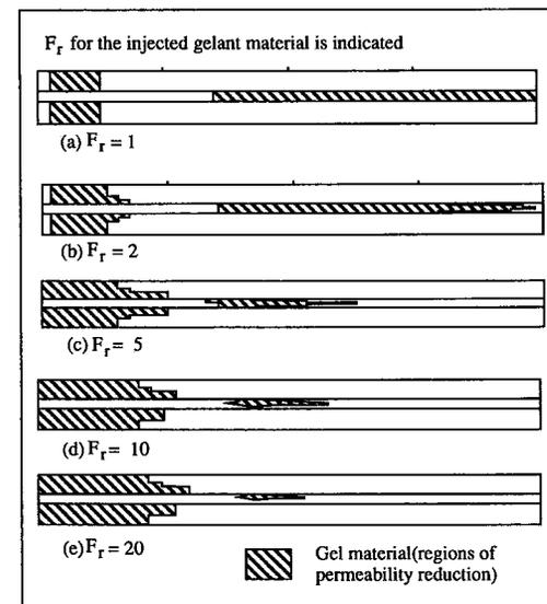
Figure 12: Calculated position of the gelant from numerical simulation for a simple three layer system with  $k_1/k_2 = 10$  for a range of gelant viscosities; 0.2 PV viscous slug followed by 0.1 PV of brine postflush. Region of reduced permeability (see text) is shown shaded.
