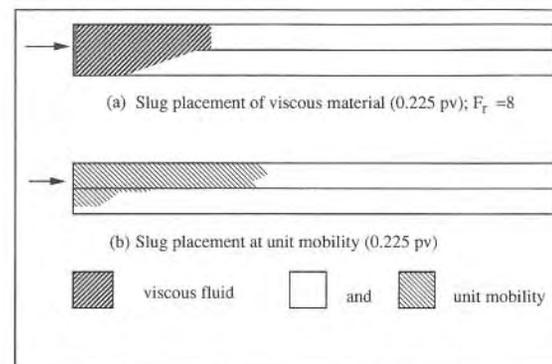
Figure 3: Comparison of (a) a viscous overstable slug placement with (b) a unit mobility case in a two layer stratified bedpack;  $k_1/k_2 = 5$ ;  $F_r = 8$  (Pack1; Table 1)
